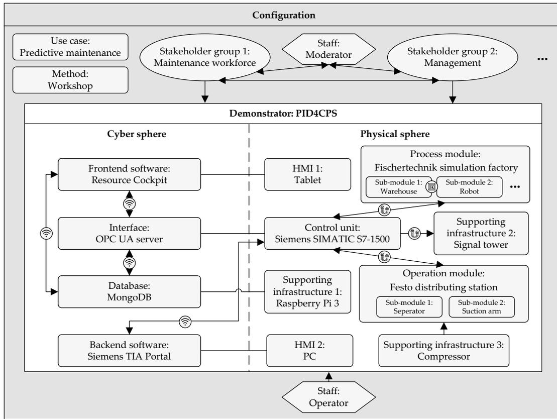
Fig. 3. Configuration of the demonstrator PID4CPS.
