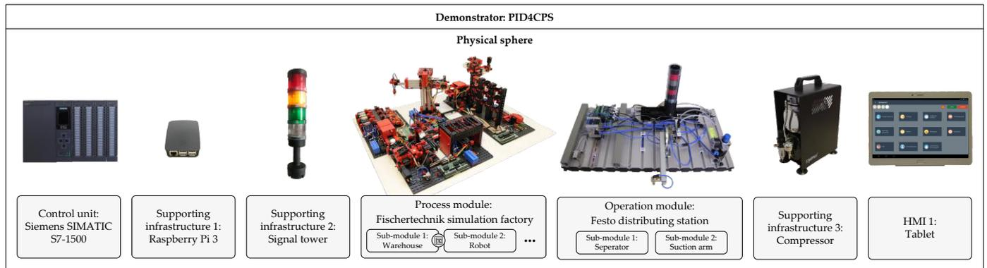
Fig. 4. Physical modules of the demonstrator PID4CPS.
